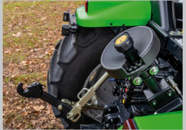
External lift controls make for easy coupling of implements.
